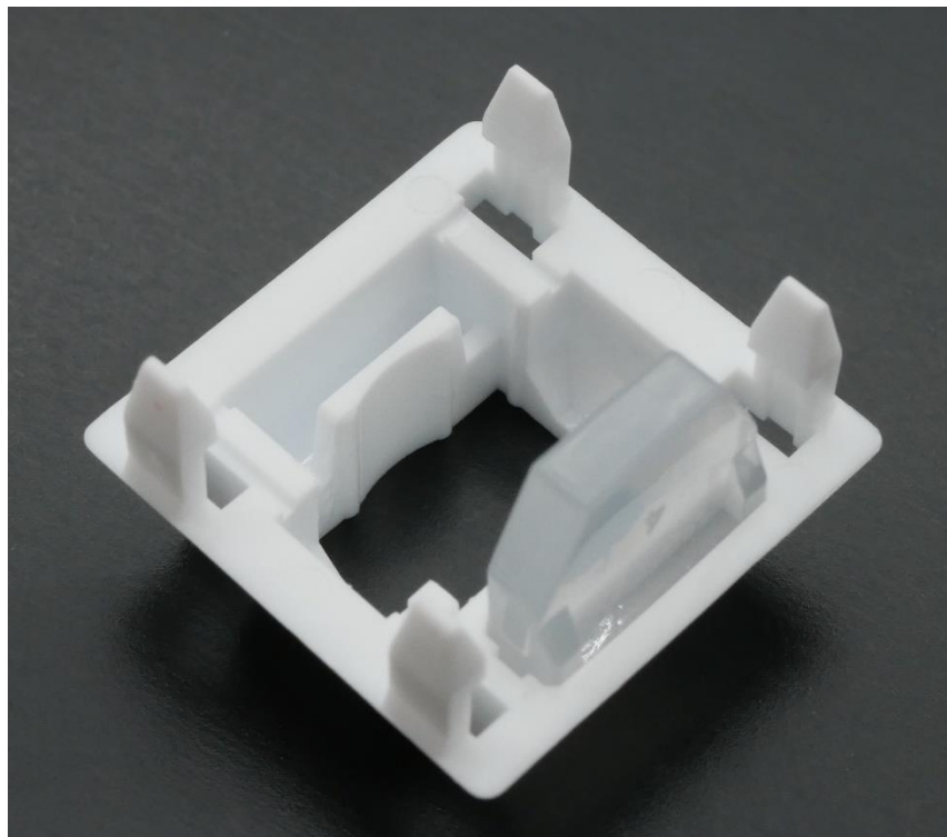
Figure 7: WS Morandi top housing internal design showing lack of distinctive mold markings and mold ejector circles around upper rim.
