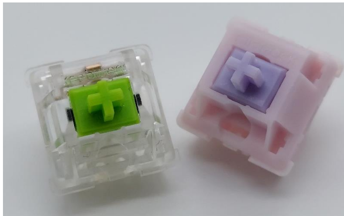
Figure 15: A rubbery silent tactile on the left in Keebwerk Tacit V1s and a plasticky linear switch on the right in Konpeitous.
