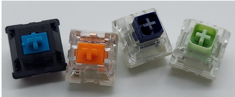
Figure 12: Comparative clicky switch scale of 'low pitched' to 'high pitched' going left to right. (L-R: Cherry MX Blue, Novelkeys x Kailh Sherbet, Kailh Box Navy, Kailh Box Jade)
