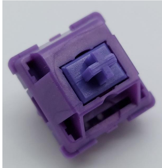
Figure 16: A Durock/JWK Taro Ball switch - one of the rare few in which I've identified this 'grinding' phenomena.
