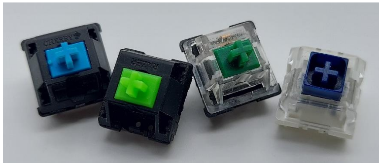
Figure 9: Comparative clicky switch scale of 'quiet' to 'loud' going left to right. (L-R: Cherry MX Blue, Greetech Chroma Razer Green, Gateron Green, Kailh Box Navy)
