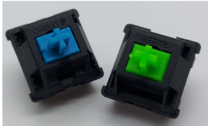
Figure 14: A pair of notoriously rattly clickjacket switches. Left is a Cherry MX Blue, Right is a Kailh Razer Green.
