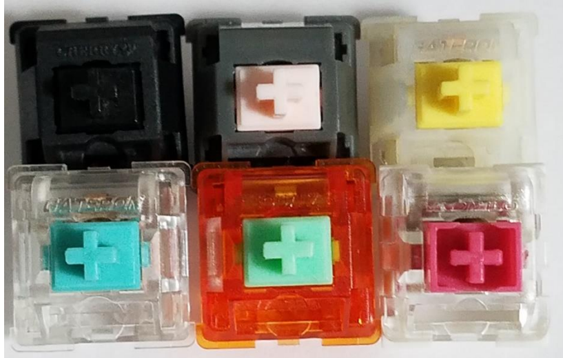
Figure 5: Switches for comparison. (L-R, Top-Bot: Cherry MX Black, Alpaca V1, Gateron Milky Yellow, Tealio V2, C3 Tangerine V2 (62g), and Varmilo EC V1 Rose)
