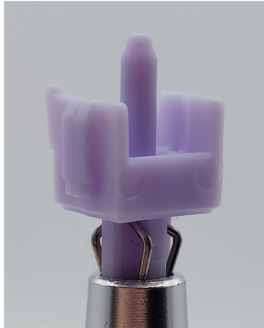
Figure 5: Konpeitou stem showing angled slider rails and large backplate mold circles.
