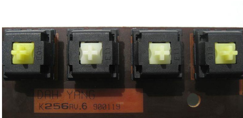
Figure 6: Variation in Yellow Jet Axes soldered within board. (Photo from Deskthority)
