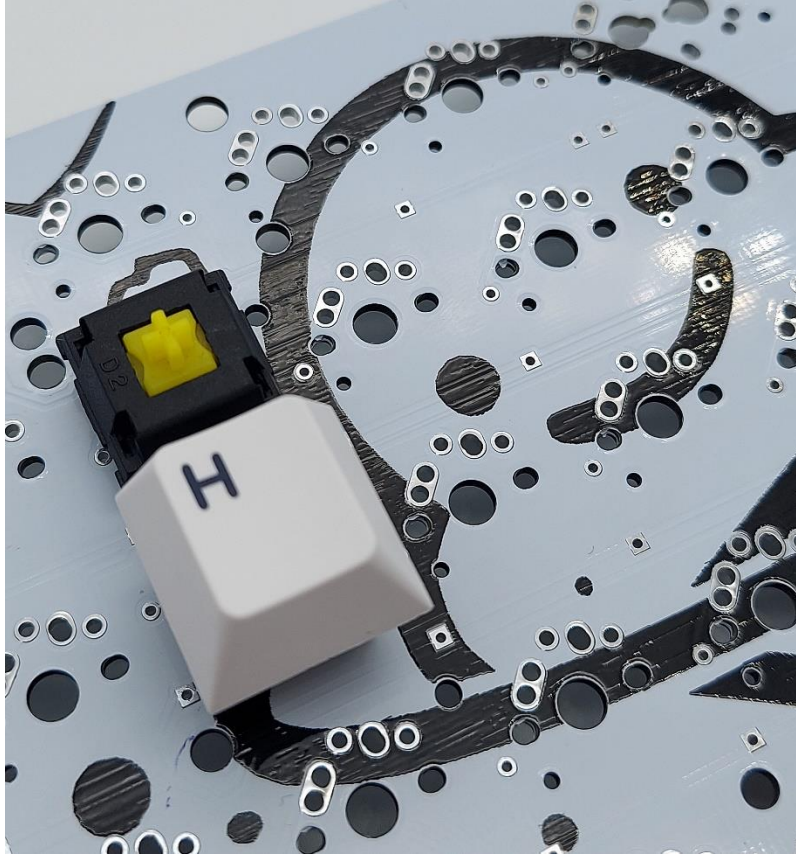
Figure 3: Taiwan Jet Axis with and without keycap in a prototype Spacey PCB from VanillaKeyboards.
