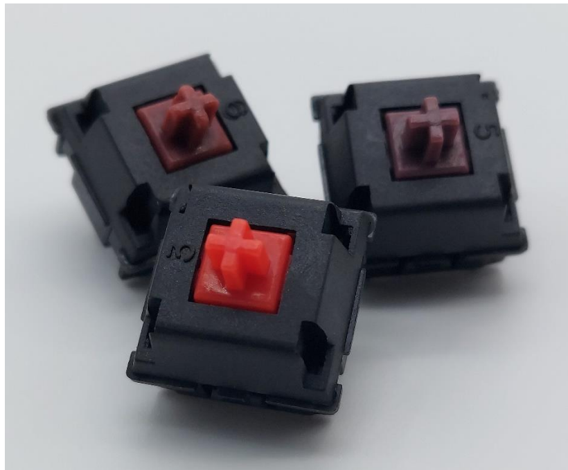
Figure 7: Variation in Red/Brown switches desoldered from the same board.
