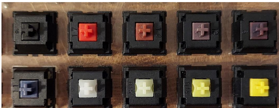
Figure 5: All known color variants of Taiwan Jet Axis switches as of time of publishing.
