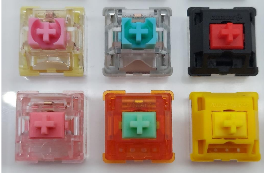
Figure 14: Switches for comparison. (L-R, Top-Bot: TTC Gold Pink, Momoka Frog V3, Cherry MX Red, KTT Strawberry, C3 Equalz Tangerine V2, Gateron Cap Yellow V2)
