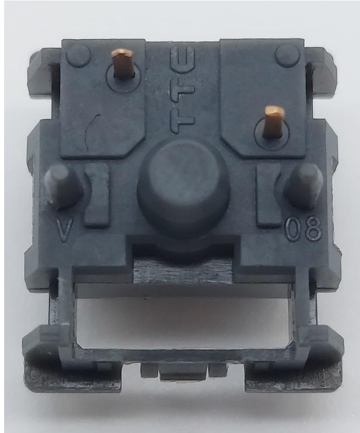
Figure 10: TTC Wild bottom housing underside showing mold markings and anticounterfeit marking.
