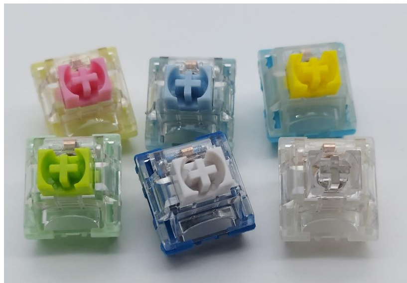
Figure 5: Family photo of dustproof switches from the modern TTC Era. (L-R, Top-Bot: Gold Pink, Blueish White, Skylar, Ace, Speed Silver, Ice)
