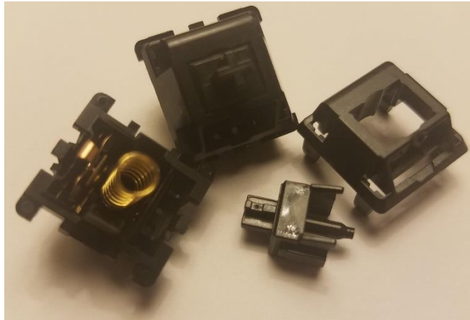
Figure 12: The bottom housings of H1s are currently the only switch to date to have 'Polyamide' plastic rather than Nylon.
