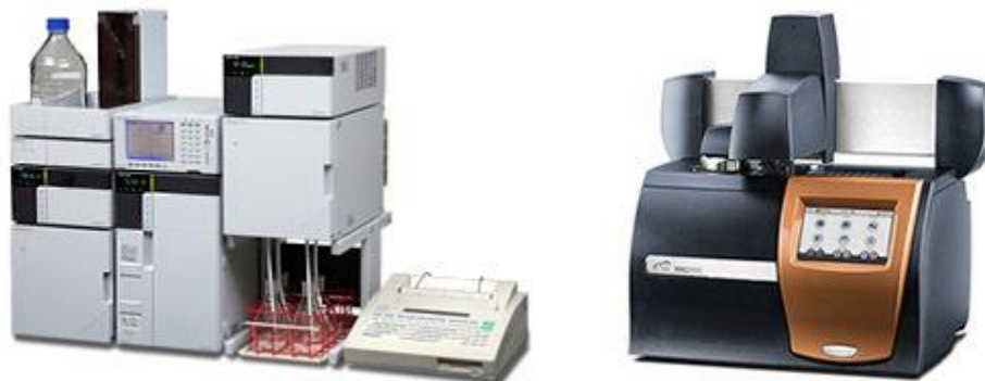
Figure 3: Pictures of a Shimadzu GPC (Left) and TA Instruments DSC (Right). These two are, in fact, the models that I worked on during my time in a rheology lab. [4,5]
