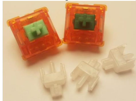
Figure 11: Picture of the only two switch pieces containing UHMWPE to date: C 3 Equalz Tangerine V2s and Invyr UHMWPE stems.
