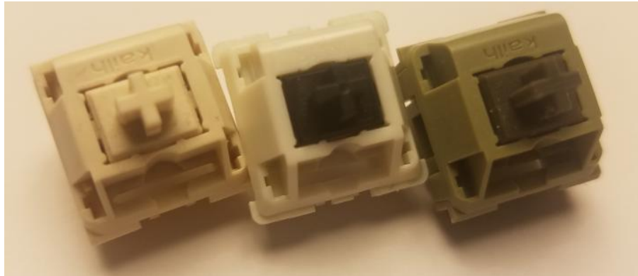
Figure 5: Notable switches featuring POM including Novelkeys Creams, Invyr Panda V3s, and Nolives (Left to Right).
