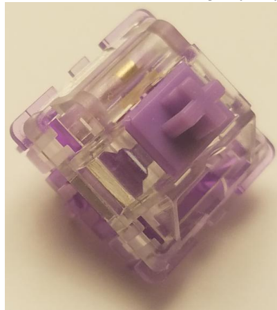
Figure 14: Everglide Crystal Purples being the only switch to date to supposedly be made of ABS plastic.
