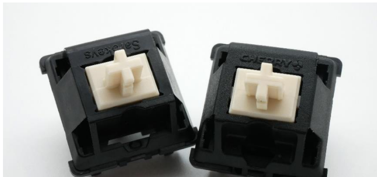
Figure 5: Visual external comparison between Sarokeys BCP switch (Left) and original Black Cherry Pie frankenswitch (Right).
