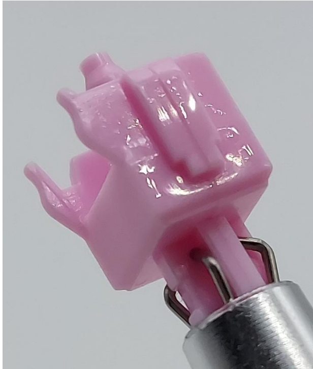
Figure 11: Total coverage of side of stem with factory lubing as can be seen by the shining of the lube against LED light.
