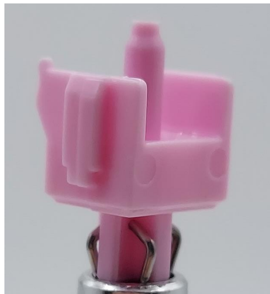
Figure 9: Angled shot of SP Star Magic Girl stem showing center pole and slider rail taper, mold circles, and pronounced transverse seam.
