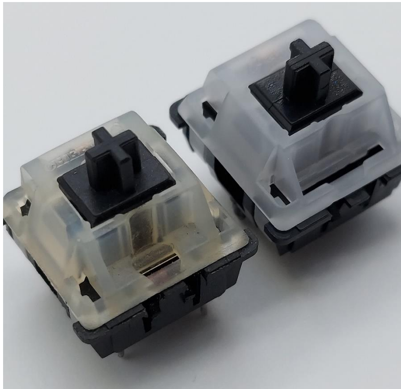
Figure 5: Top-down view of Nixie Black switch housings (Left) and Opblack switch housings (Right).
