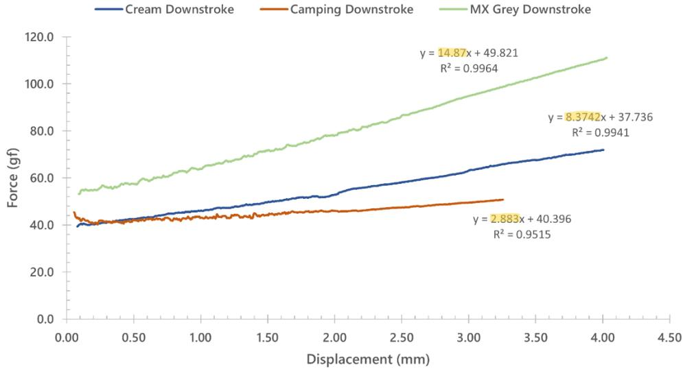
**Figure 1:** Comparison of slopes of the linear region for three different switches with equations for line of best fit included. Note that the highlighted values correspond to the 'Slope' discussed above.
