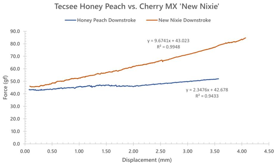
**Figure 3:** Isolated linear region of downstroke force curves for Tecsee Honey Peach and Cherry MX 'New Nixie' switches with equations for line of best fit through each curve.
