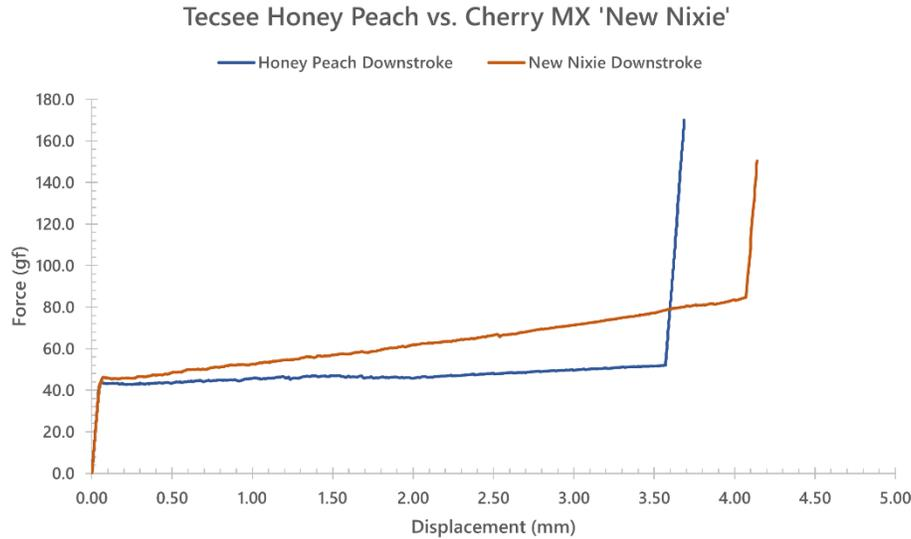
**Figure 2:** Isolated downstroke force curves for Tecsee Honey Peach and Cherry MX 'New Nixie' switches.
