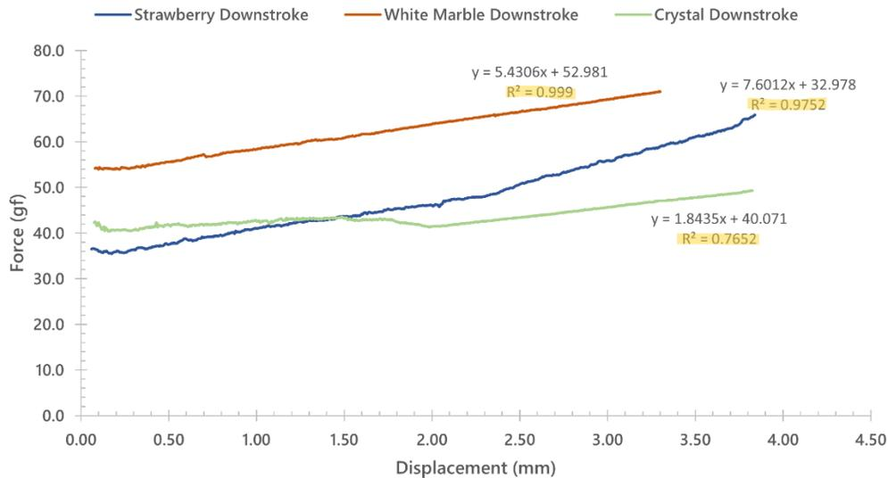
**Figure 5:** Comparison of flatness of the linear region for three different switches with equations for line of best fit included. Note that the highlighted values correspond to the 'Linearity' discussed above.
