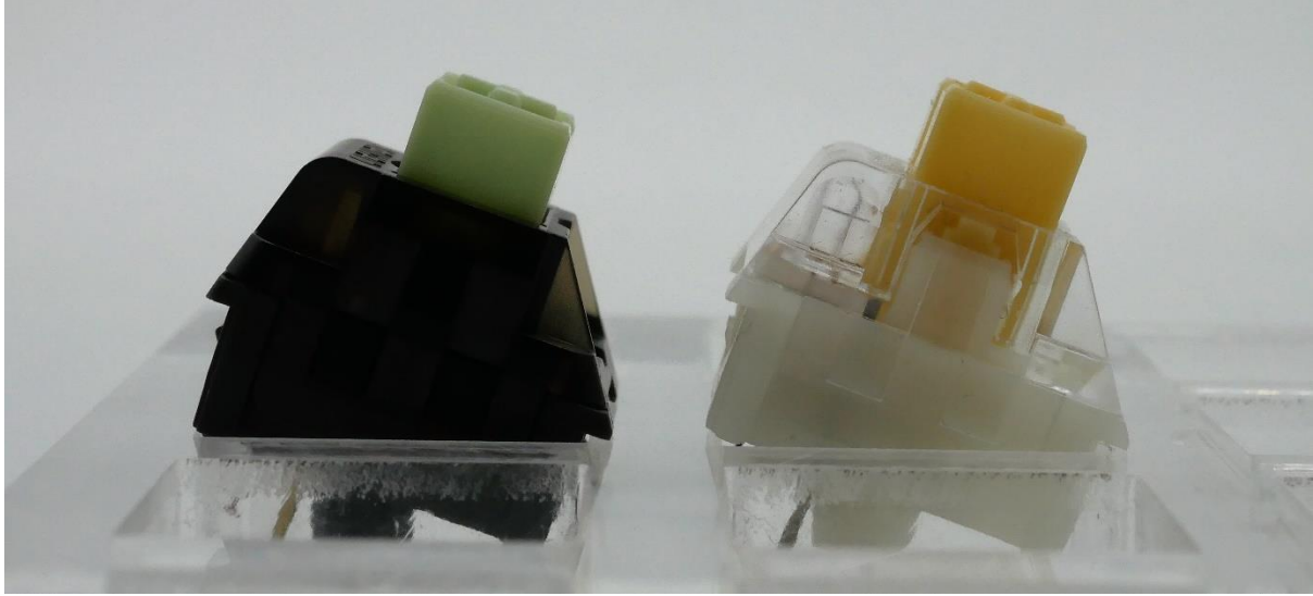
Figure 3: LICHICX Green Mustard and Varmilo EC Daisy V2 side profile showing identical general shape and protrusion of keycap mounting stem above the dustproof stem walls.
