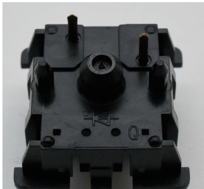
Figure 8: Obsidian L bottom housing external design showing single capital letter mold marking between 3rd and 4th LED/Diode pins.
