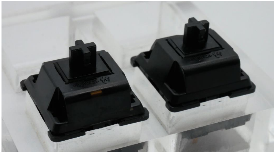
Figure 6: Obsidian Pro V2 (Left) top housing translucency as compared to the Obsidian L (Right) opacity.
