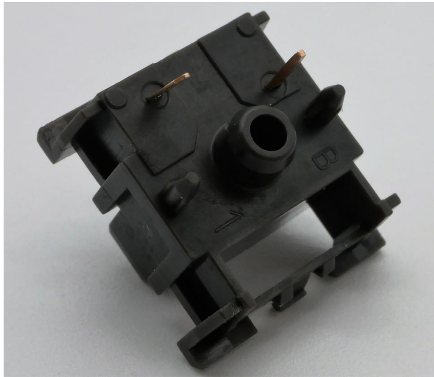
Figure 12: Novelkeys Cream Clickie bottom housing exterior showing wide open LED slot, sideways mold markings, and hollowed center mast.
