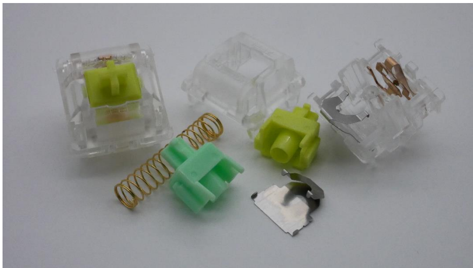
Figure 2: Zeal 3-in-1 Clickiez switches and their components.
