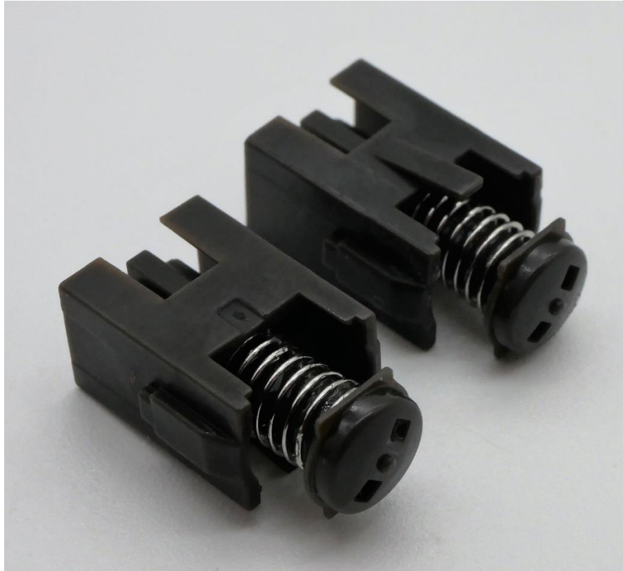
Figure 11: Back (Left) and Front (Right) sides of the Cream Clickie stem unit showing contained spring design and singular centered stem leg.
