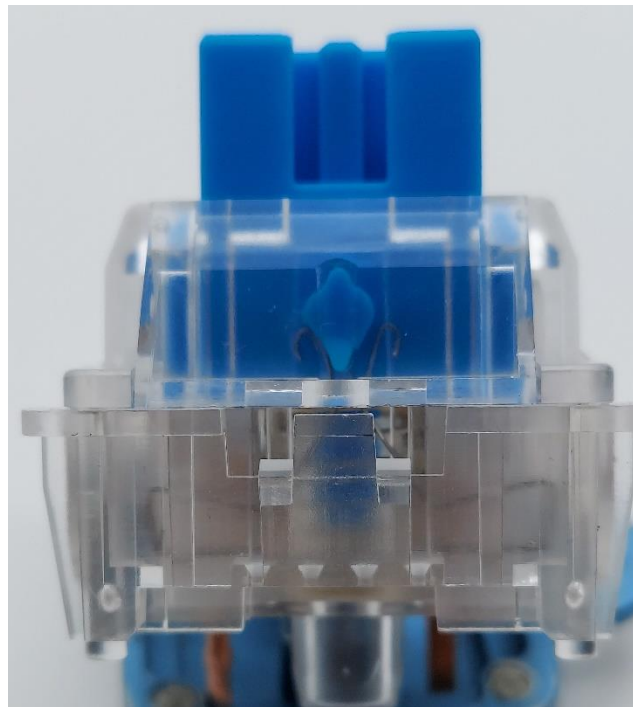
Figure 5: Snap spring mechanism located within a large GTMX Blue switch.
