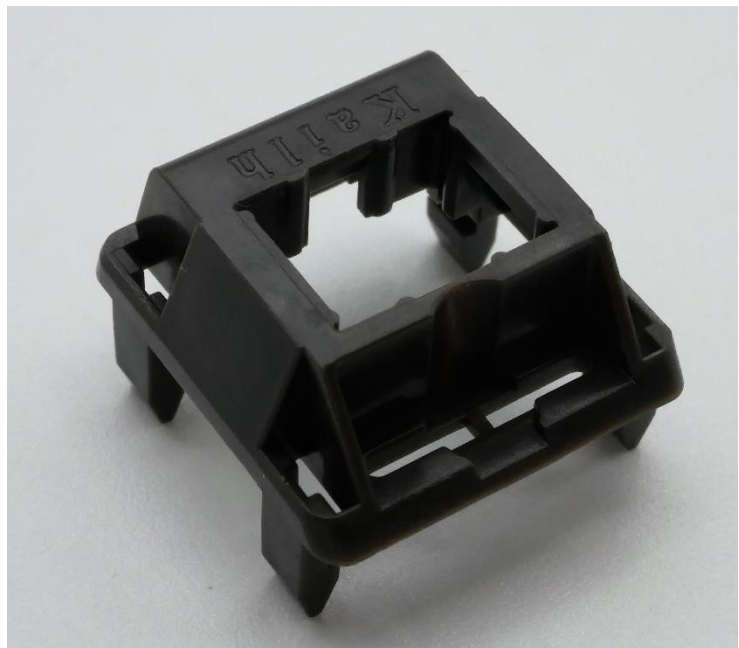
Figure 9: Novelkeys Cream Clickie top housings showing inverted, old 'Kailh' nameplate and bifurcated LED slot.
