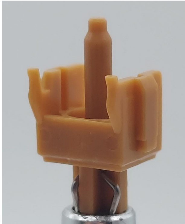
Figure 7: Angled Neapolitan stem shot showing the center pole taper, angled slider rails, and front-set mold circles.
