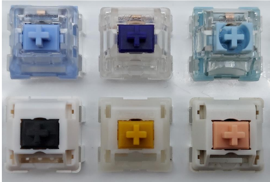
Figure 12: Switches for comparison. (L-R, Top-Bot: Kailh Polia, Zealio V2 (78g), TTC Blueish White, Moyo Black, Gazzew U4T, Invyr Holy Panda)
