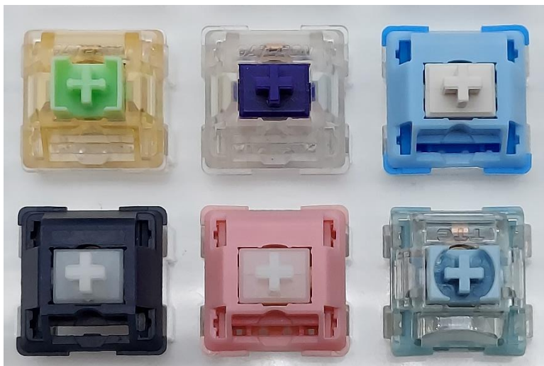
Figure 10: Switches for comparison. (L-R, Top-Bot: Gateron Kangaroo Ink, Zealio V2 (67g), Penguin, Naevy V1 (POM), Okomochi V2, TTC Blueish White)
