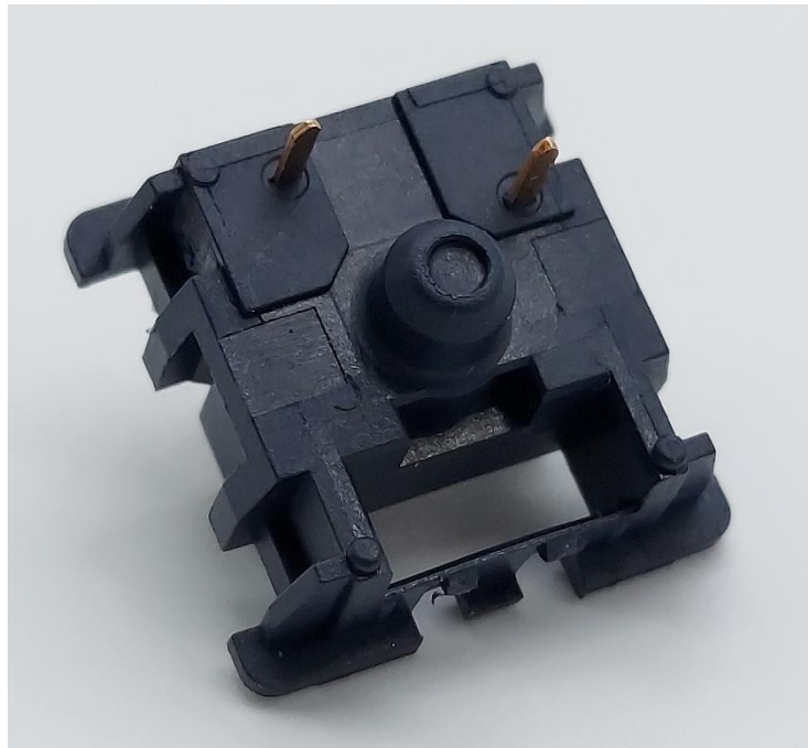
Figure 9: Bottom of Naevy bottom housings with rectangular regions.
