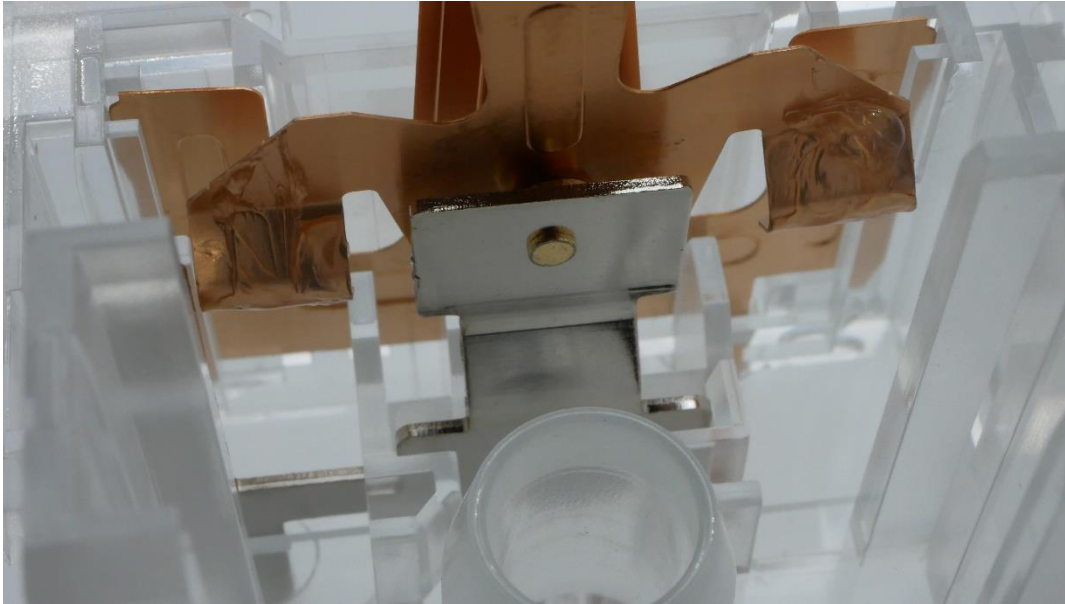
FIGURE 9: NOVELKEYS X KAILH BIG DARK YELLOW BOTTOM HOUSING INTERIOR SHOWING MASSIVE LEAVES WITH FACTORY LUBRICANT.
