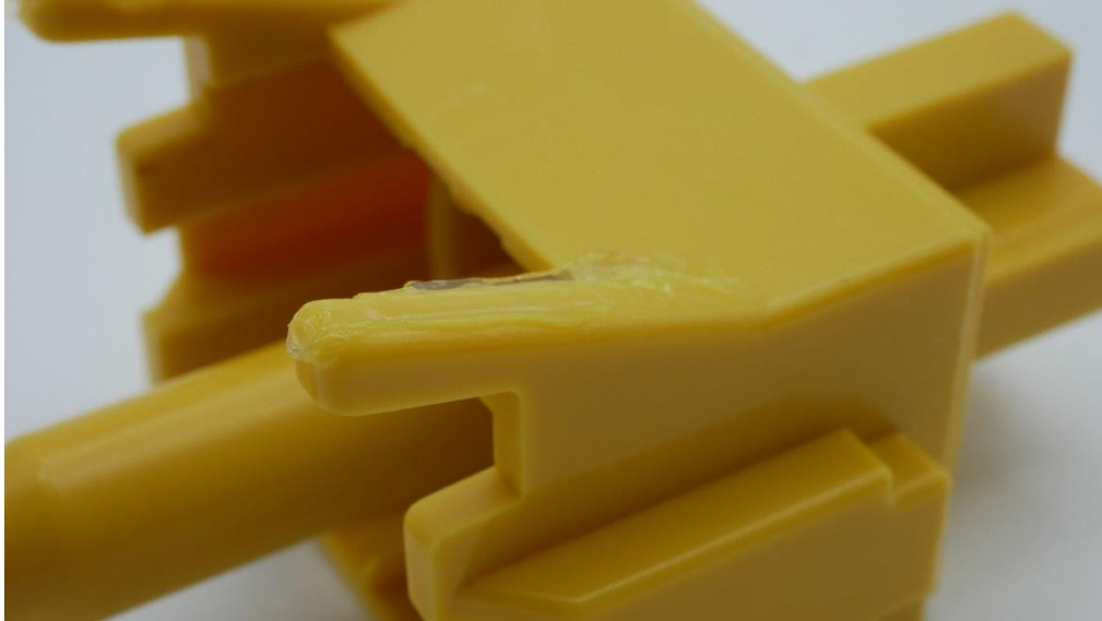
FIGURE 8: THICK FACTORY LUBING ON THE STEM LEGS OF THE NOVELKEYS X KAILH BIG DARK YELLOW SWITCH.
