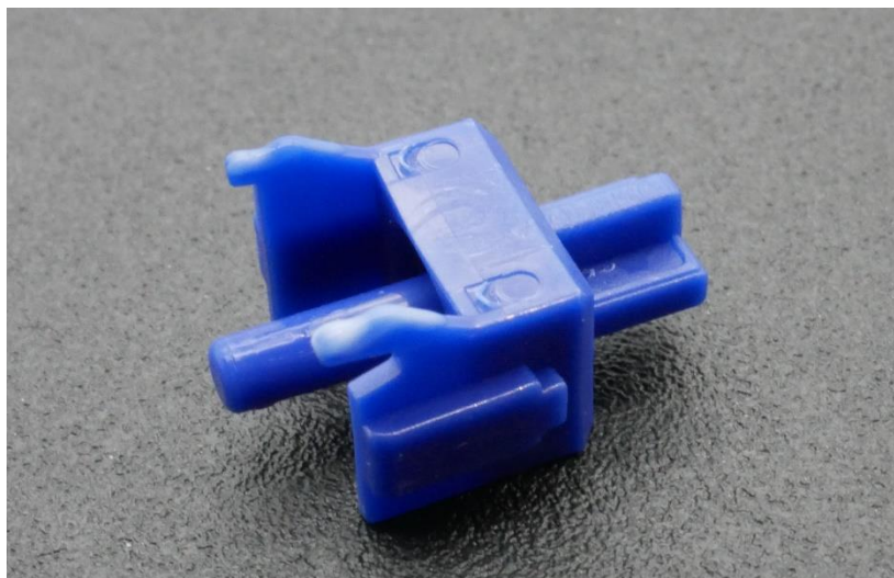
Figure 12: Momoka Shark stem front side showing non-uniform mold ejector circles, front plate seam, and factory lubrication on stem legs.
