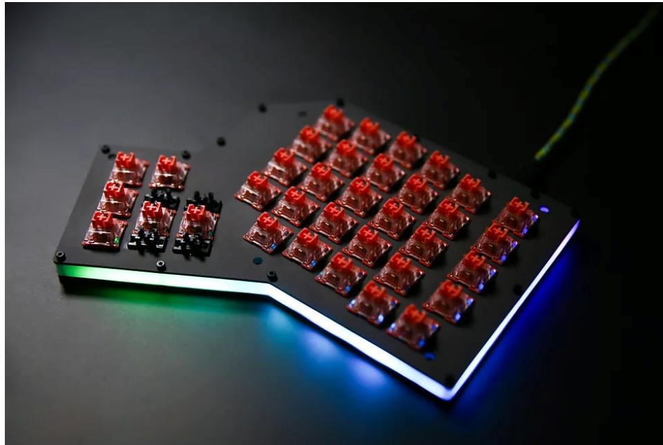
Figure 7: Half of a Momoka Ergo keyboard with Flamingo switches preinstalled.
