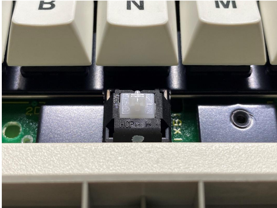
Figure 3: HCP Hirose Clear switch with ink marking denoting its use as a spacebar.
