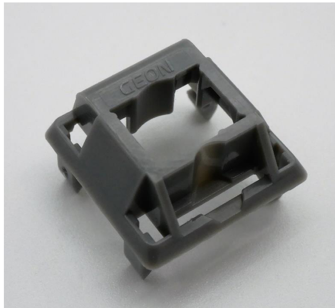
Figure 8: Lubed Black Geon switch top housing externals showing rectangular LED slot and stylized 'GEON' nameplate.
