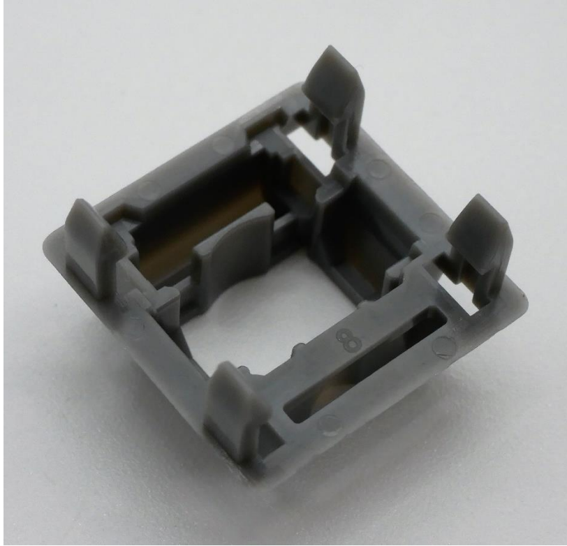
Figure 11: Lubed Black Geon switch top housing internals showing centered, single number mold marking next to LED slot.
