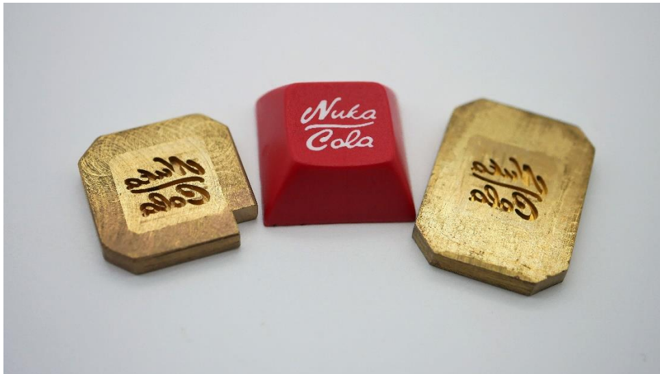
Figure 1: Original SP DSA (Left) and SA (Right) molds from the 2014 Geekhack run.
