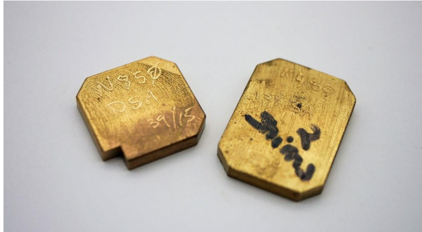
Figure 2: Backside of the DSA (Left) and SA (Right) Nuka Cola molds showing manufacturing inscriptions.
