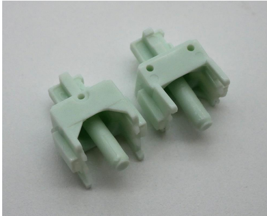
Figure 14: Gecko stem front and backplates showing sloped edges and extra sets of through-switch holes with unknown functionality.
