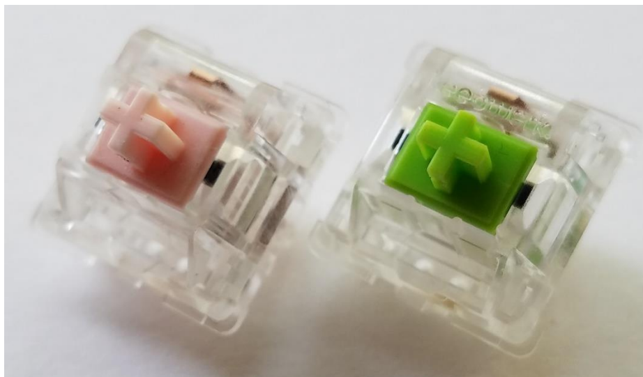
Figure 4: Picture of Durock factory sample for the Ghost silent linear switch (left) and Keebwerk Tacit switch (right).
