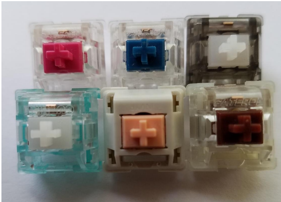
Figure 5: Switches for comparison. (L-R, Top-Bot: Aliaz 70g, Zilent V2 67g, Everglide Oreo, Outemu U4 Silent Tactile 68g, Massdrop x Invyr Holy Panda, Gateron Silent Brown)
