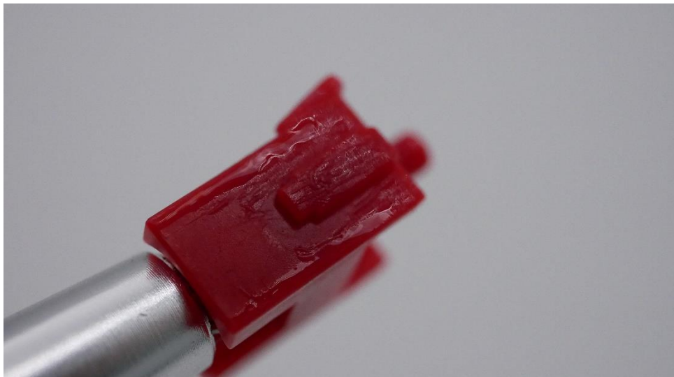
Figure 12: Kailh Christmas Tree stem showing stock factory lubrication and non-tapered slider rail.
