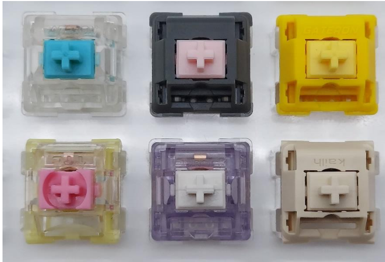
Figure 12: Switches for comparison. (L-R, Top-Bot: Tealio V2, Alpaca V2, Gateron Cap Yellow, TTC Gold Pink, Lavender, Novelkeys Cream)
