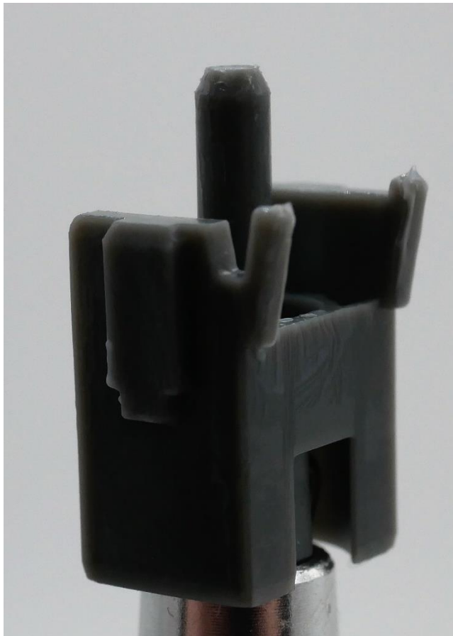
Figure 11: Alternative angle of Invokeys Black Sesame stem showing factory lubrication on front plate and slider rails.
