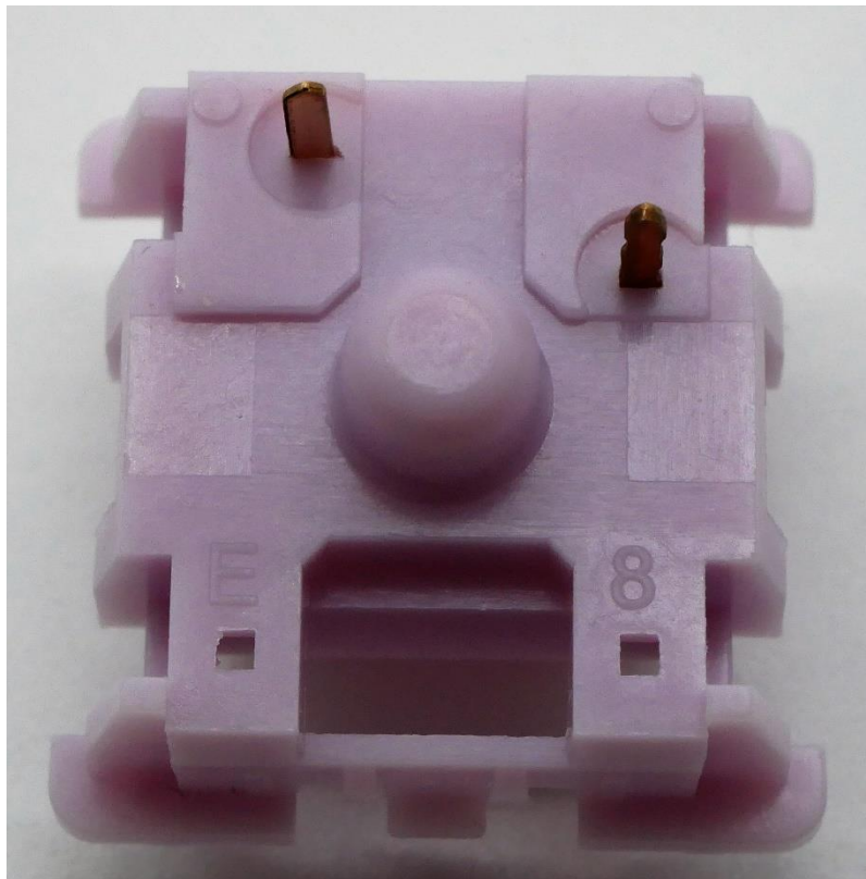
Figure 12: Huano Fi bottom housing external design showing three pin construction and two different mold markings near diode pin holes.
