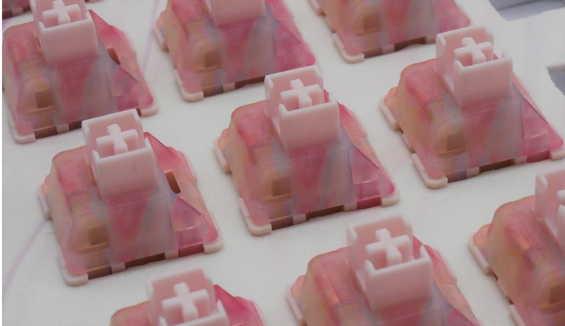
Figure 10: Overflow color swirl pattern present in Huano Hi switches which also shows the repetition of pattern location and size across numerous switches.
