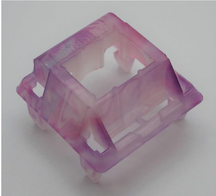
Figure 8: Huano Fi top housing exterior showing inverted 'HUANO' nameplate and thin, bifurcated LED slot design.
