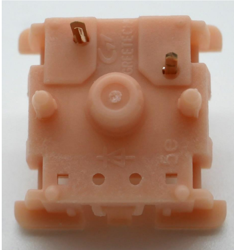
Figure 8: Greetech Sunset bottom housing exterior design showing 5-Pin construction, mold marking in lower right hand corner, and 'Greetech' logo in between metal PCB pins.
