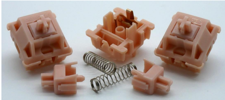
Figure 5: Greetech Sunset switches and their components.
