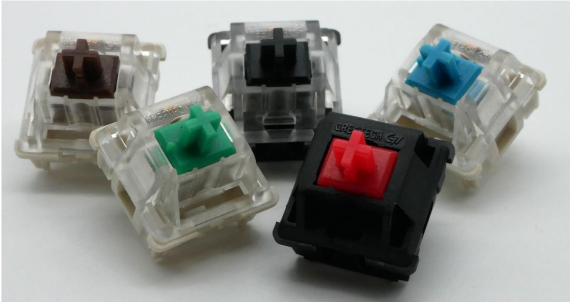
Figure 3: A representative portion of my Greetech OEM switch collection showcasing the different stem colors and housing combinations made over the years.
