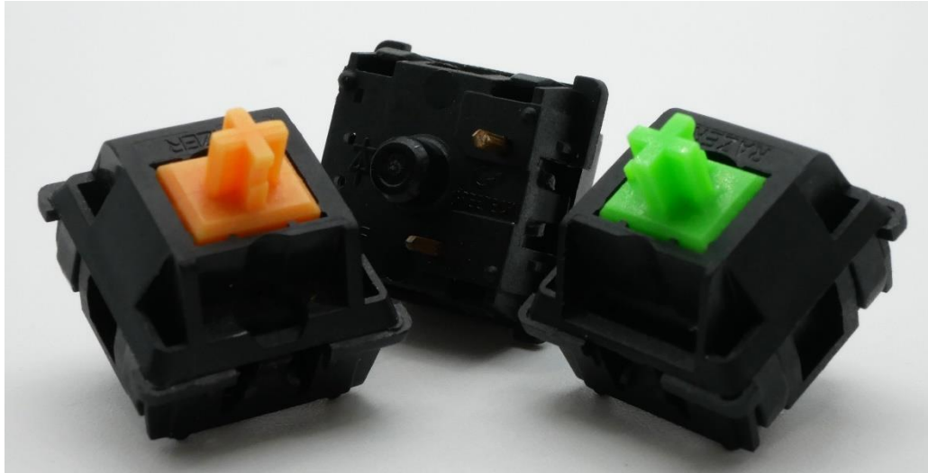
Figure 4: Greeotech Razer switches with the Razer Yellow upturned to show Greeotech marking on bottom housing exterior.
