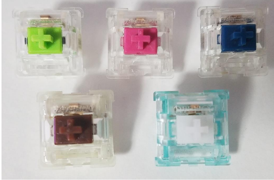
Figure 6: Switches for comparison. (L-R, Top-Bot: Keebwerk Tacit V1, Aliaz 80g, Zilent V2 67g, Gateron Silent Brown, Outemu Sky Silent Tactile 68g)
