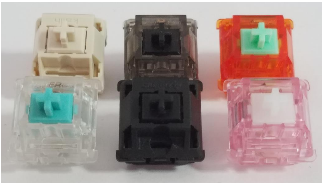
Figure 12: Switches for comparison. (L-R, Top-Bot: Novelkeys Cream, Gateron Ink V2, C3 Tangerine V2 (62g), Tealios V2, Cherry MX Black, Pinoko V2)
