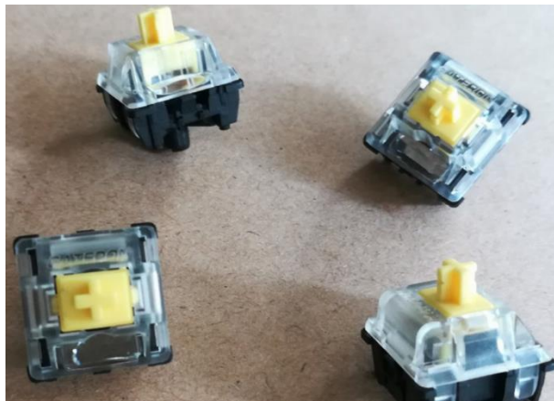
Figure 10: Gateron Optical Yellow KS-15s. Note the lack of pins on the switch in the top left.
