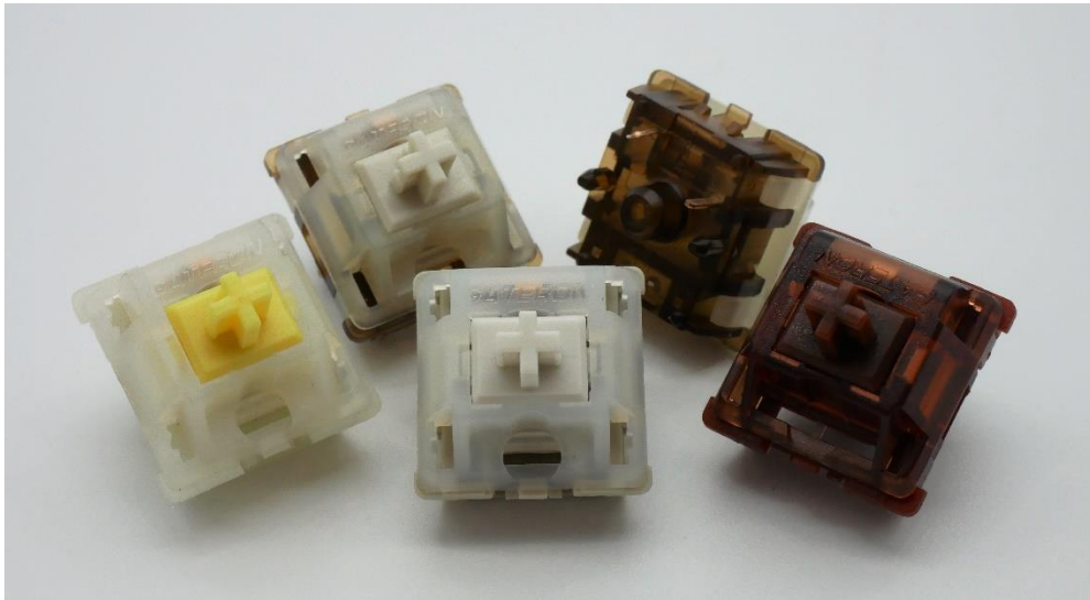
Figure 7: Color comparison between Gateron Root Beer Float (Back) and Gateron Milky Yellow (Left), Gateron X V2 (Middle), and Keychron Phantom Brown (Right).
