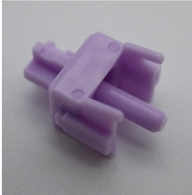
Figure 7: Gateron Mink stem showing mold ejector circles, non-tapered slider rails, and lightly tapered central pole.
