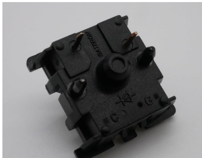
Figure 14: Gateron Mink bottom housing external design showing pair of single letter mold markings in LED pin-out region, PCB mount pins, and GATERON anticounterfeit stamp.
