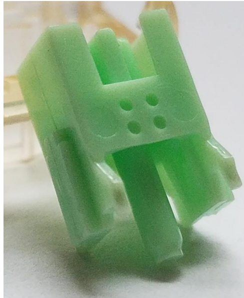
Figure 5: Dots on the front side of Gateron Kangaroo Ink stems.
