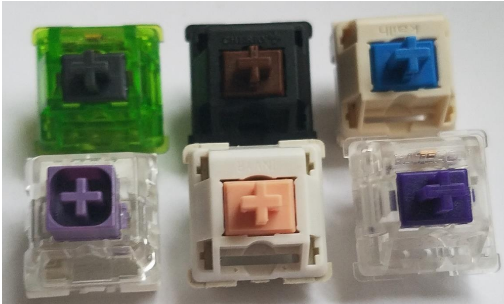
Figure 9: Switches for comparison. (L-R, Top-Bot: C3 Kiwi, Cherry MX Brown, Novelkeys Blueberry, Kailh Box Royal, Massdrop x Invyr Holy Panda, Zealio V2 68g)
