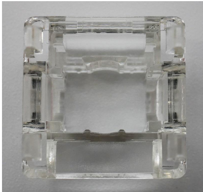
Figure 10: Gateron G Pro 3.0 Yellow top housing interior design showing single letter/digit mold markings in upper left- and right-hand corners.
