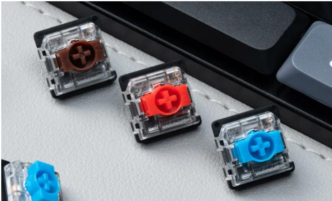
Figure 6: Gateron KS-27 low profile Brown, Red, and Blue switches. Note that the KS-33s outwardly appear near identical to the KS-27s.
