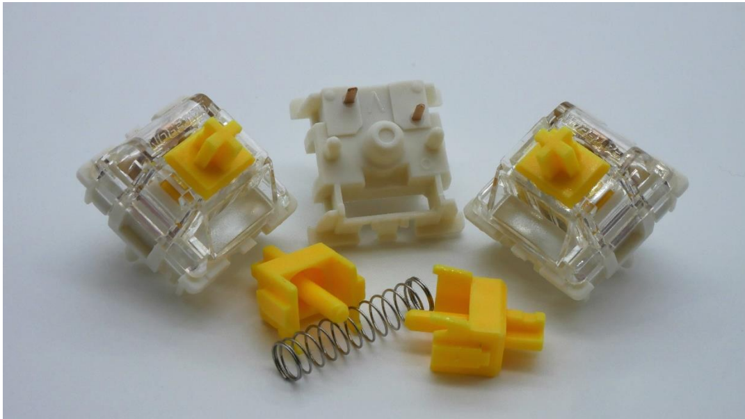
Figure 9: Gateron G Pro 3.0 Yellow switch and its components.
