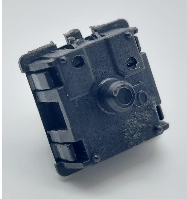
Figure 3: Interestingly as well, the stabilizer switch did not come with a leaf in it at all. (Contrast increased to better show bottom side design features.)
