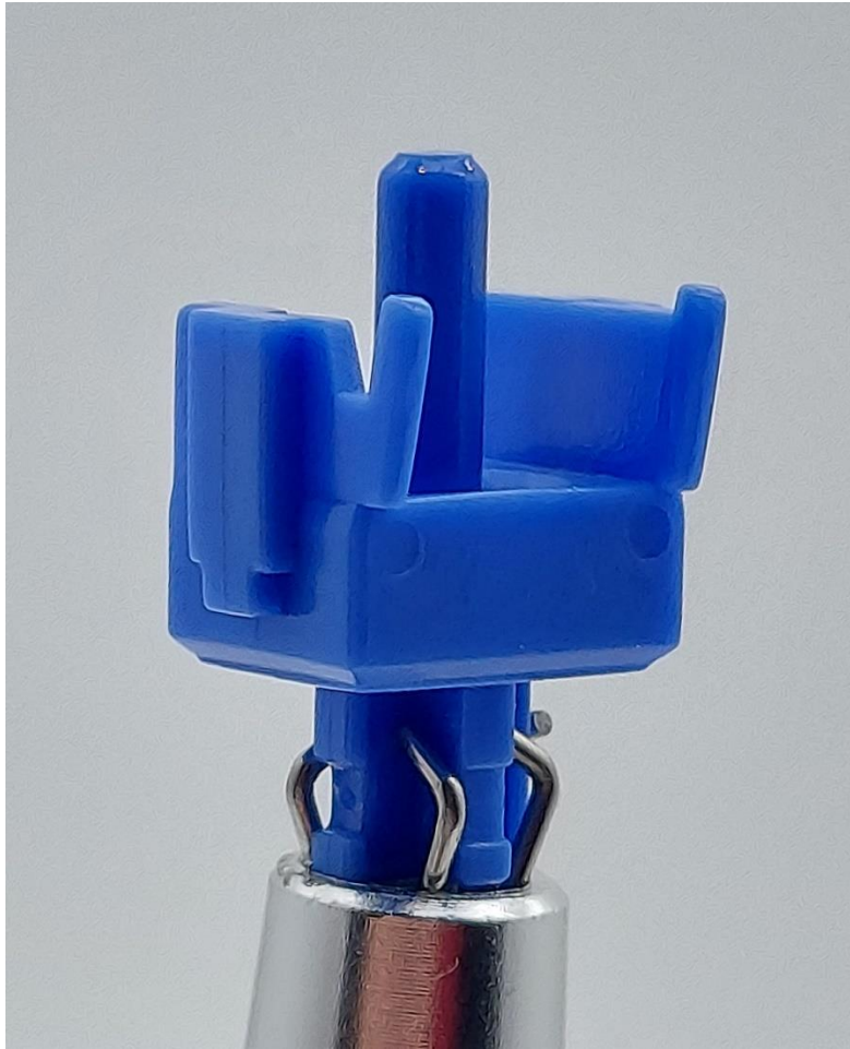
Figure 6: Gateron CJ stem wide shot showing slightly tapered central pole, squared off slider rails, and medium, wide set mold circles.
