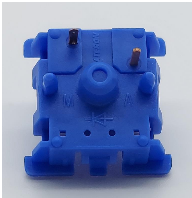
Figure 10: CJ bottom housing external design demonstrating mold markings and 'GATERON' anticounterfeit mold marking.
