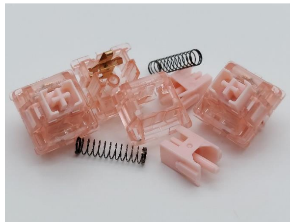
Figure 6: Gateron Box Ink Pink components with black, stock springs.
