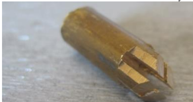
Figure 10: Picture of one of the few 'stem shaver' tools designed for fixing old Box switch stems.
