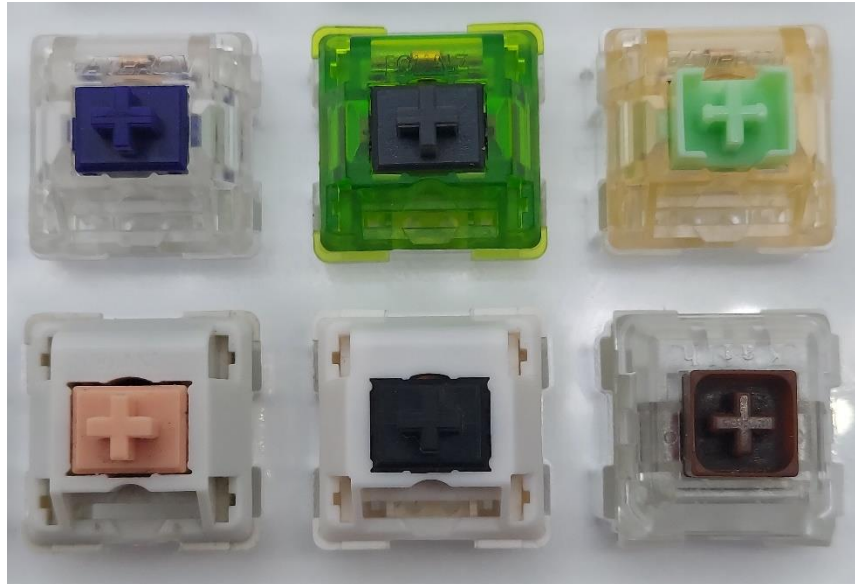
Figure 18: Switches for comparison. (L-R, Top-Bot: Zealio V2 (78g), C3 Kiwi, Gateron Kangaroo Ink, Massdrop x Invyr Holy Panda, Moyu Black, Kailh Box Brown)
