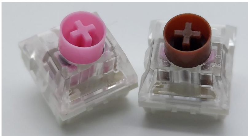
Figure 6: Kailh Box Silent Pink and Box Silent Brown switches with the new rounded off stems.
