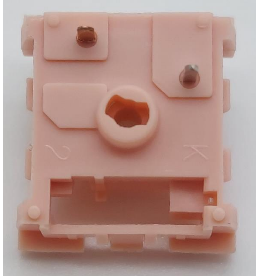
Figure 14: Reinforcement patch on bottom side of Novelia bottom housings.
