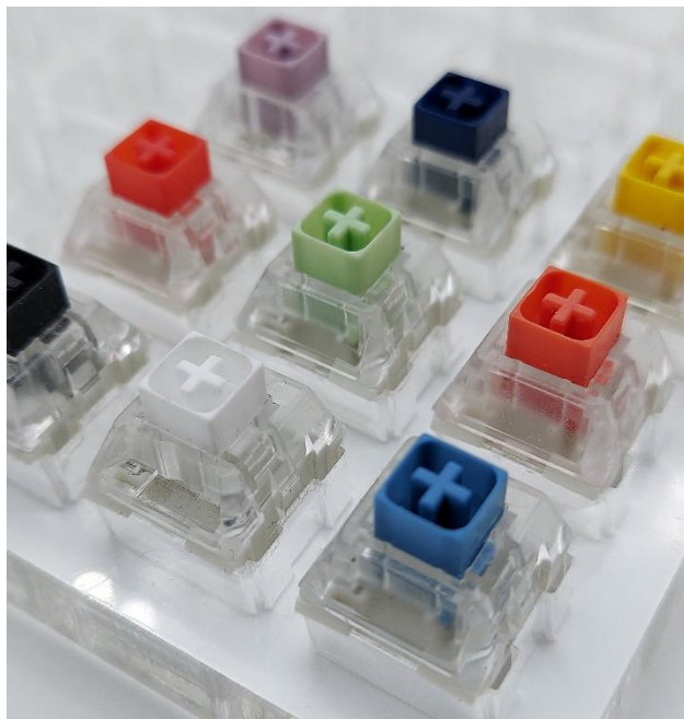
Figure 5: A small sampling of ‘traditional’ Box switches available at the time of writing.
