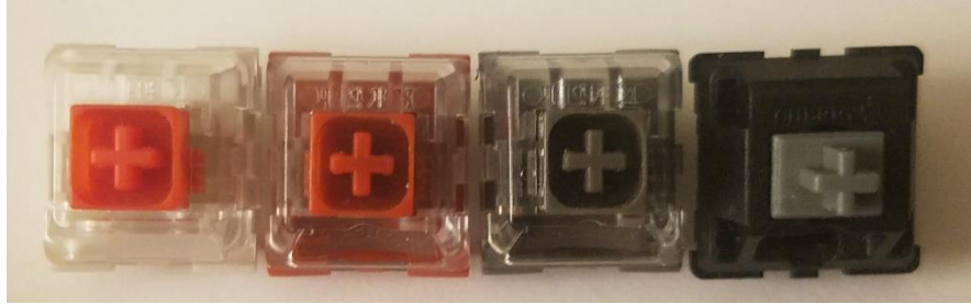
Figure 3: Linear switch color comparisons. (Left to Right: Kailh Box Red, Box Chinese Red, Box Ancient Grey, Cherry MX Grey)
