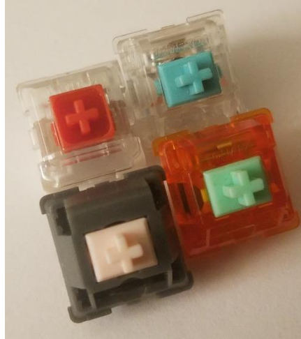
Figure 6: Switches used for comparison. (L-R, Top-Bot: Kailh Box Red, Tealio V2, Alpaca, C 3 Tangerine V2 62g.)
