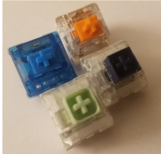
Figure 7: Switches used for comparison. (L-R, Top-Bot: Novelkeys Sherbet, Gateron Ink Blue, Kailh Box Navy, Kailh Box Jade)
