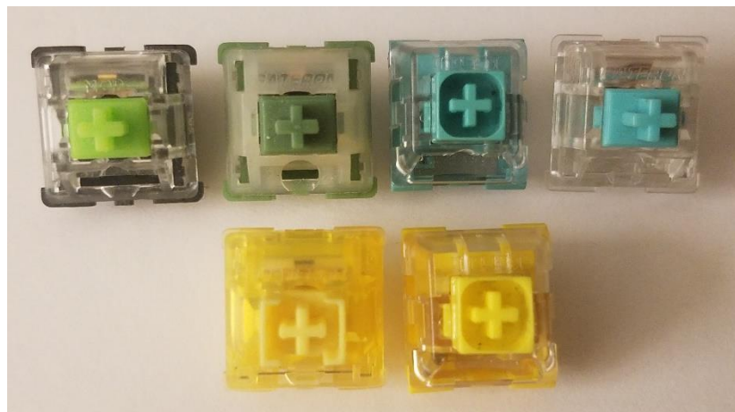
Figure 4: Clicky switch color comparisons. (L-R, Top-Bottom: MOD-SH, FEI Matcha V1, Box Glazed Green, Tealio V2, Gateron Ink Yellow, Box Noble Yellow)
