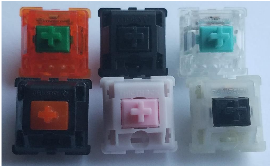
Figure 8: Switches for comparison. (L-R, Top-Bot: C3 Tangerine V2 (67g), Cherry MX Hyperglide Black, Tealio V2, Cherry Hirose Orange, ThicThock Marshmallow V1, Gateron Milky Black)
