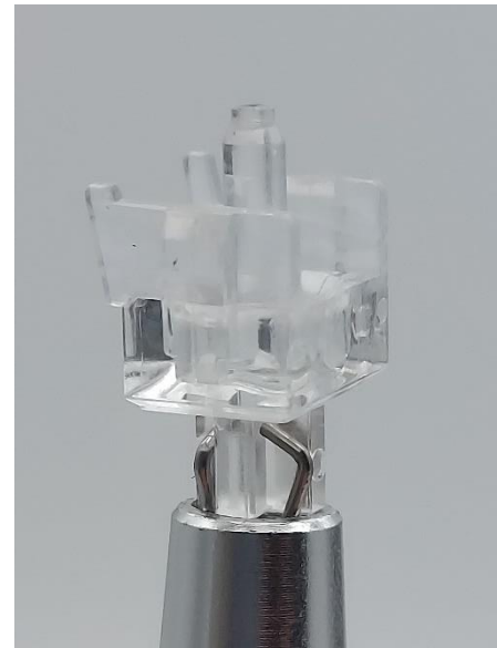
Figure 11: Picture of Everglide V3 stem which shows factory lube application as a function of the difference in clarity across the stem.
