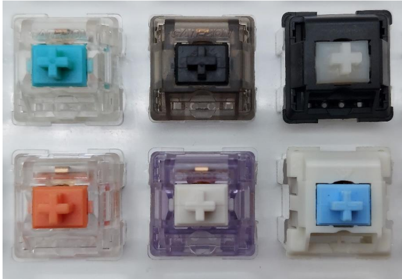
Figure 13: Switches for comparison. (L-R, Top-Bot: Tealio V2, Gateron Black Ink V2, Durock POM Linear, Everglide Amber Orange V2, Lavender, KTT Cloud Blue)
