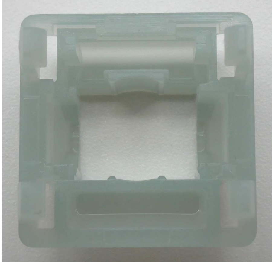
Figure 9: Everfree Grayish Tactile top housing interior design showing capital letter mold markings in upper left- and right-hand corners.
