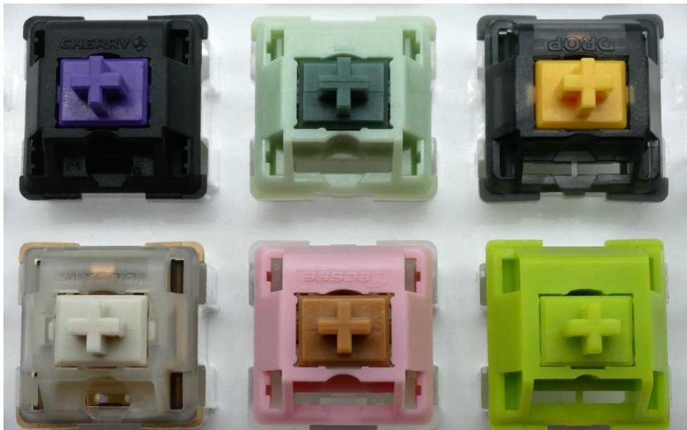
Figure 20: Switches for comparison. (L-R, Top-Bot: Cherry MX Purple, Zaku II, Drop Holy Panda X, Gateron Root Beer Float, Neapolitan Ice Cream, and KTT Matcha)
