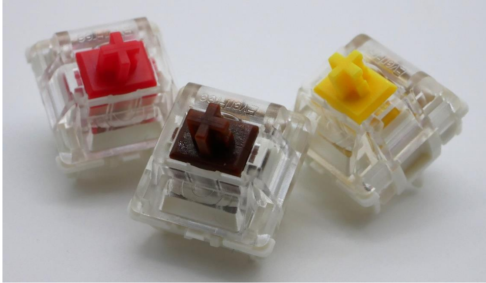
Figure 5: Original Everfree OEM trio featuring unique LED diffuser design front and center.
