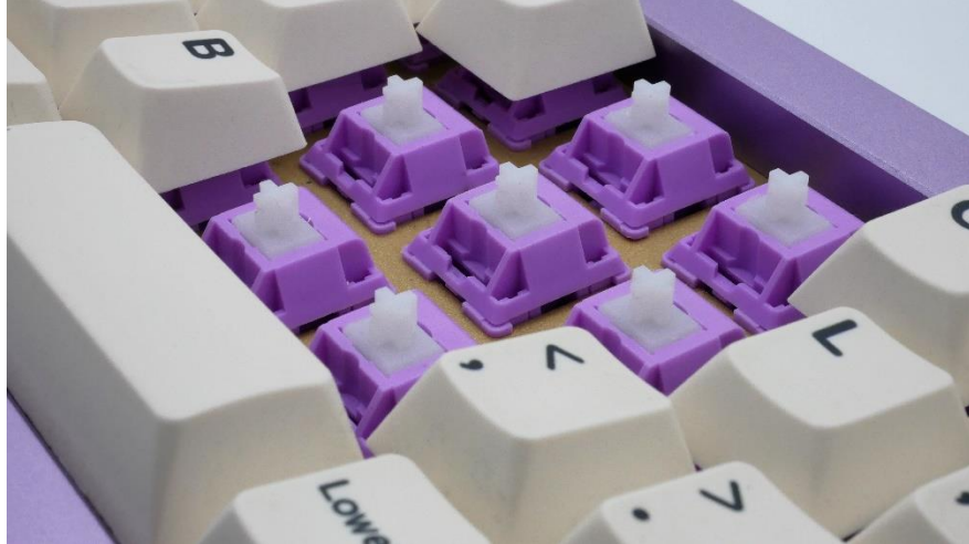
Figure 2: And there they are - stock EMT V1s in all of their scratchy scratchy glory.
