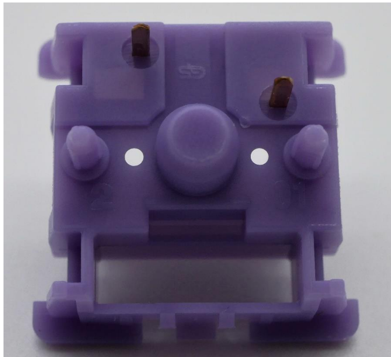
Figure 14: EMT V2 bottom housing external design showing 'GS' and numerical mold markings as well as rings around the PCB mounting pings indicative of Haimu.
