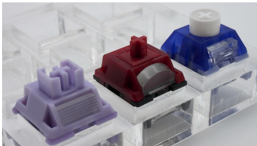
Figure 10: LED diffuser shape and design comparison between Haimu (Purple), TTC (Red), and Kailh (Blue).
