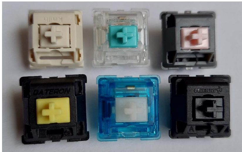
Figure 7: Switches for comparison. (L-R, Top-Bot: Novelkeys Cream, Tealio V2, Alpaca V2, Gateron KS3 Yellow, Original Aspiration, Cherry MX Black)
