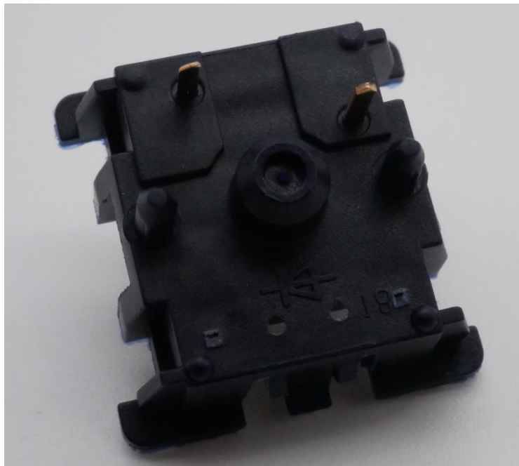
Figure 13: Designer Studio Graphite Gold bottom housing externals showing PCB mounting pins as well as double digit mold marking in bottom right-hand corner.
