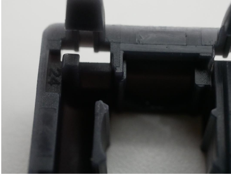
Figure 10: Zoomed in photo of the upper right-hand side double digit mold marking in the Graphite Gold switch top housings.
