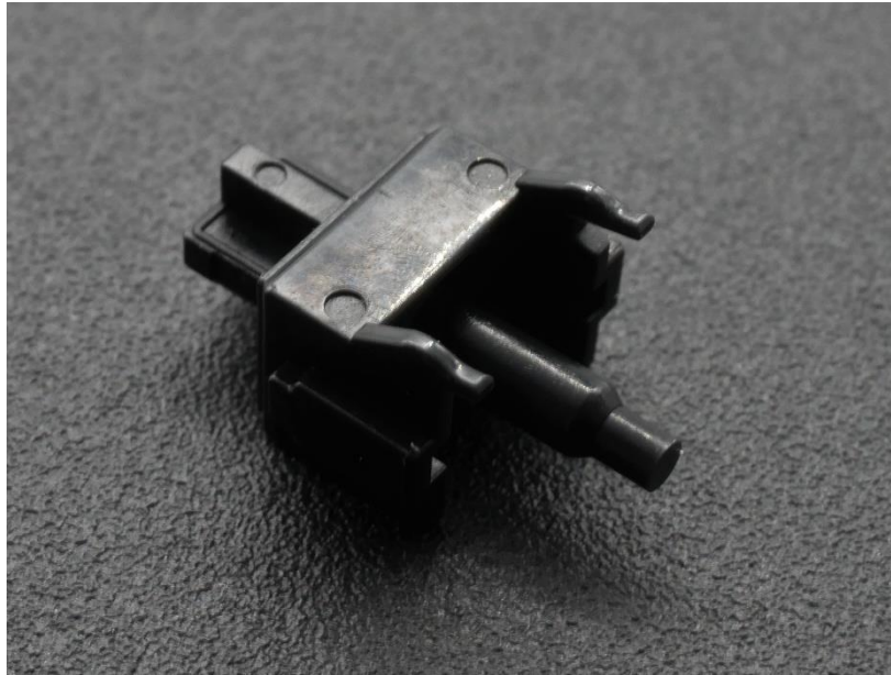
Figure 6: Cookies n' Cream stems showing non-tapered slide rails, tiered central pole, and front plate mold ejector circles.
