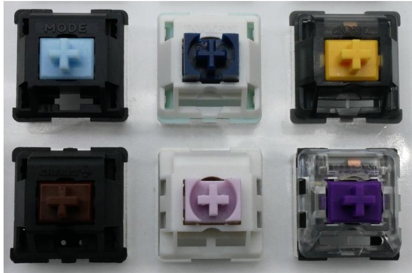
Figure 21: Switches for comparison. (L-R, Top-Bot: MODE Tomorrow, Lubed Invokeys Blueberry Chiffon, Gateron Holy Panda X, Cherry MX Brown, JWICK Taro, and Kailh Pro Purple (PCB Mount))
