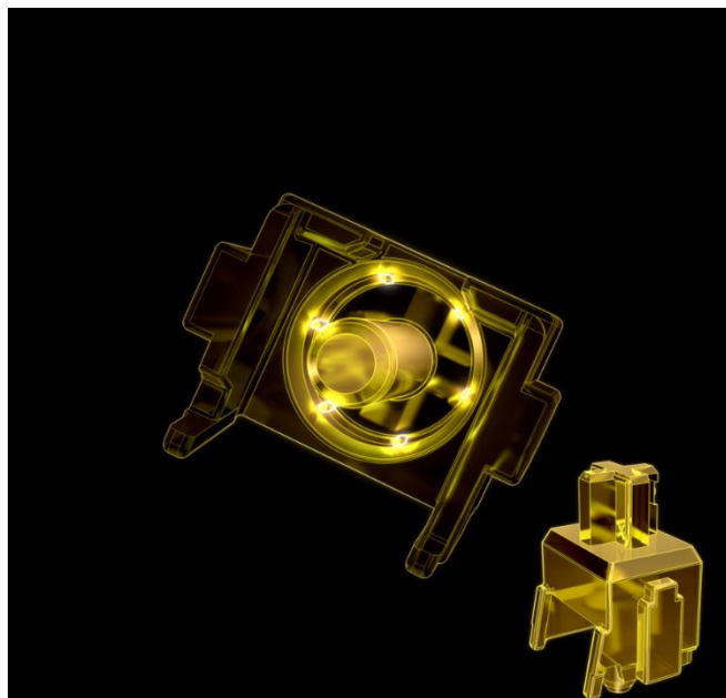
Figure 6: Introduction of stem 'crowns' in the interior of the MX2A stems as highlighted in Cherry's MX2A announcement page.
