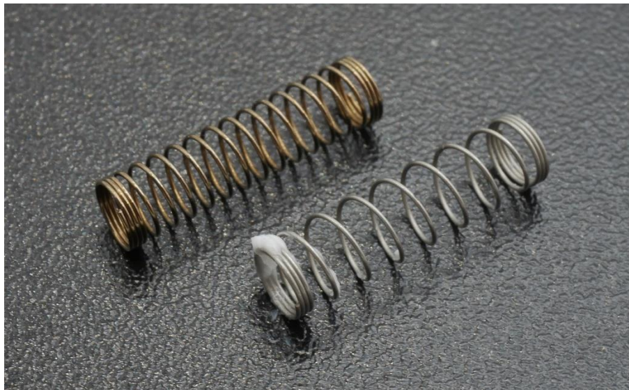
Figure 19: Unmarked comparison of Cherry MX RGB Red (Gold, Left) spring and Cherry MX2A RGB Black (Silver, Right) spring.
