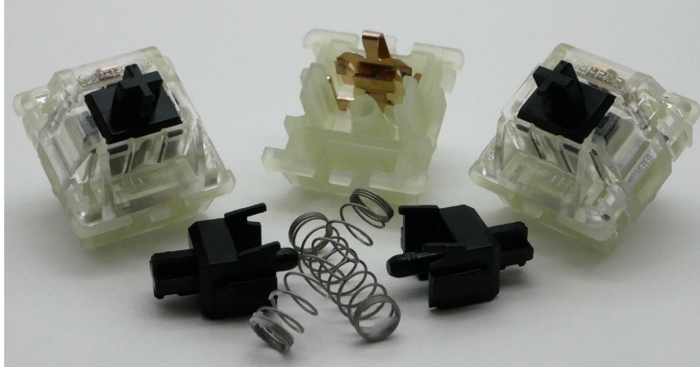
Figure 10: Cherry MX2A RGB Black switches and their components.
