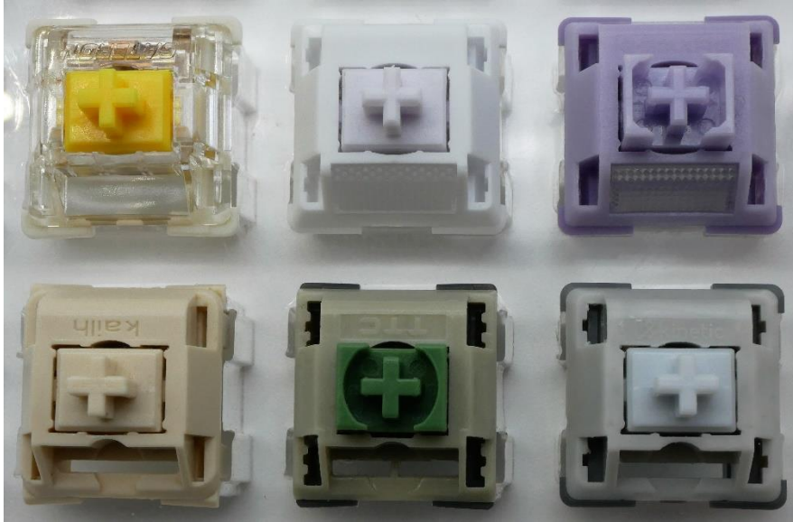
Figure 20: Switches for comparison. (L-R, Top-Bot: Gateron G Pro 3.0 Yellow, Wuque Studio Morandi, EMT V2, Novelkeys Cream, TTC Wild (42g), and Husky)
