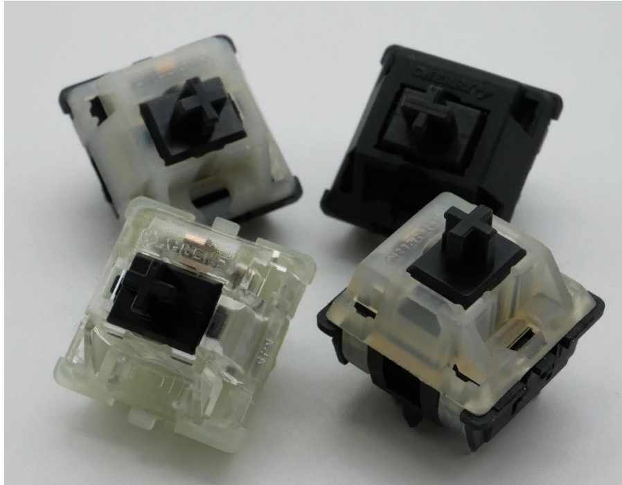
Figure 4: Cherry MX Black variation family including a 'New Nixie', OG Nixie, MX Black, and MX2A RGB Black.
