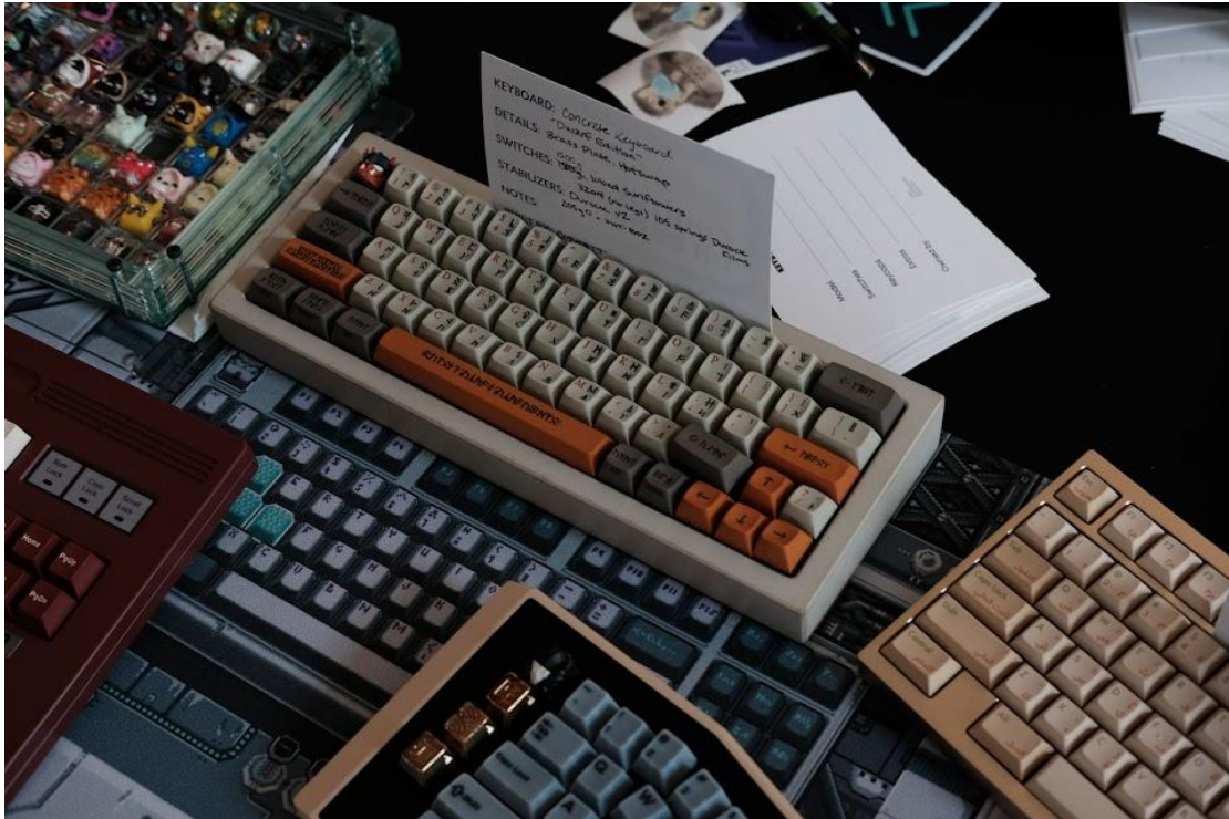
Figure 3: A concrete keyboard with 1500g switches under each key.
