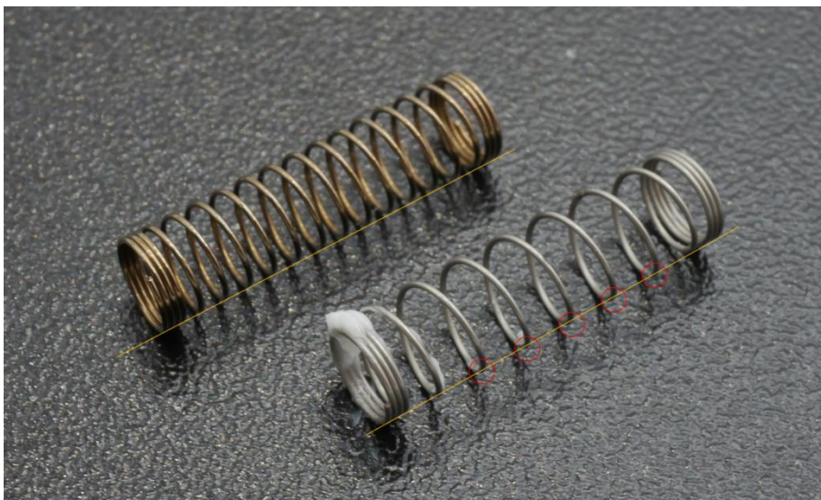
Figure 20: Marked comparison of Cherry MX RGB Red (Gold, Left) spring and Cherry MX2A RGB Black (Silver, Right) spring showing the extremely subtle bowing of the center coils in the MX2A design.
