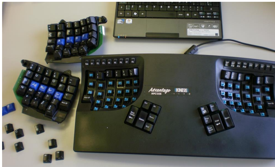
Figure 1: Kinesis Advantage 1 with Cherry MX Blue switches. [Photo from natas206 on Deskthority]
