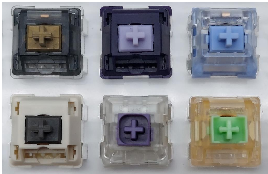
Figure 8: Switches for comparison. (L-R, Top-Bot: Pewter, Lilac, Kailh Polia, Koala, Kailh Box Royal, Gateron Kangaroo Ink)
