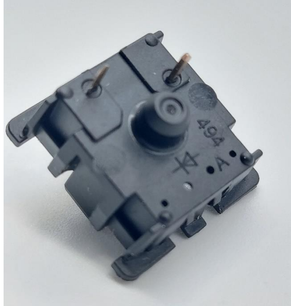
Figure 7: Cherry MX Brown bottom housing mold markings.
