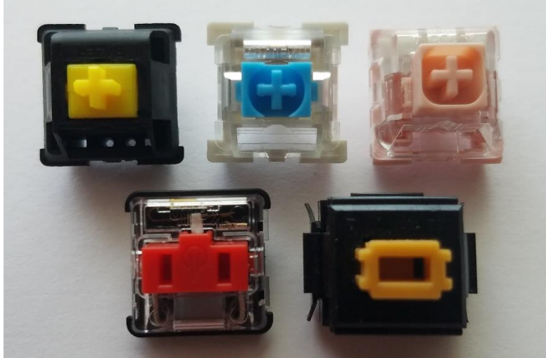
Figure 10: Different common switch mounts. (L-R, Top-Bot: Greetech Razer Yellow, Outemu Dustproof Blue, Novelia, Kailh Choc Low Profile Red, Alps SKCM Amber)
