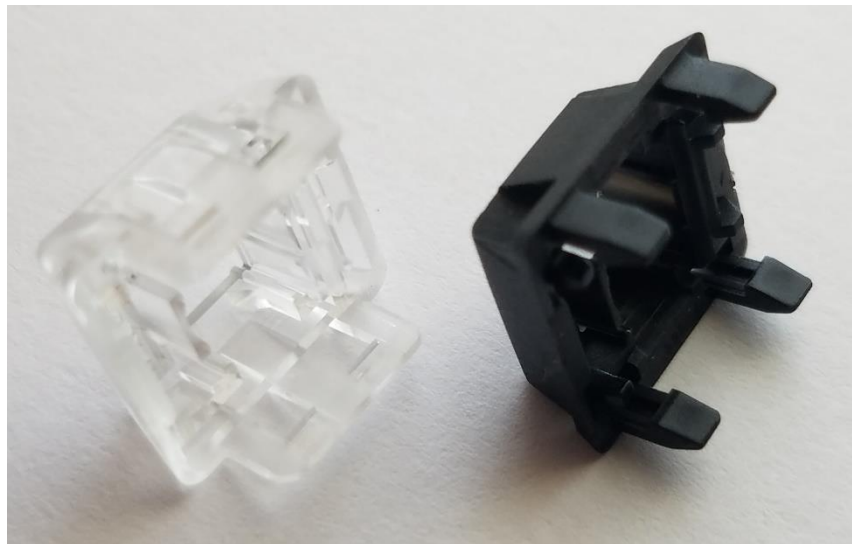
Figure 8: Winglatch style top housing (Left) compared to a 4-Pin style top housing (Right).
